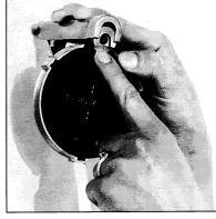
Push down on tray and insert proper shell holder.
